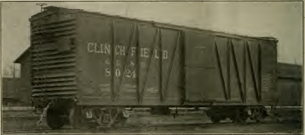
SINGLE SHEATHED BOX CAR FOR THE CAROLINA, CLINCHFIELD & OHIO RAILROAD. Bettendorf Company, Bettendorf, Iowa, Builders.
